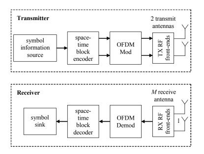
Figure 1. System block diagram.
