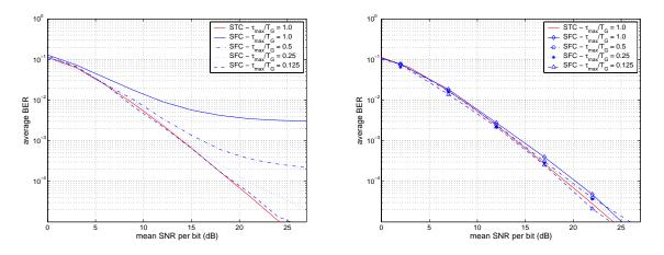
Figure 2. Alamouti-based SFC for QPSK modulation and different frequency selective transmission channels and with matched filter (left) and advanced joint maximum likelihood decoding (right).
