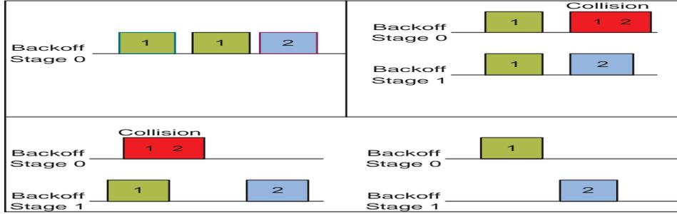
Fig. 2. Channel capture by node 1
