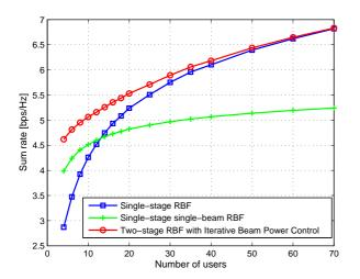
Fig. 4. Sum rate versus the number of users for Iterative Beam Power Allocation with M = 4 transmit antennas, Doppler shift  $f_D = 100$  Hz and SNR = 10 dB.
