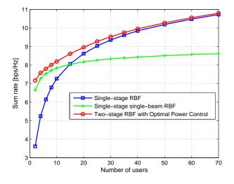
Fig. 1. Sum rate versus the number of users for Optimal Beam Power Control with M = 2 transmit antennas, SNR = 20 dB and Doppler shift  $f_D = 60$  Hz. Significant throughput gains are achieved by optimally allocating the power across beams for systems with low to moderate number of users.
