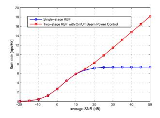
Fig. 6. Sum rate versus average SNR for On/Off Beam Power Control with M = 4 transmit antennas and K = 25 users. Interference-limited behavior (bounded sum rate) is avoided by selecting TDMA transmission mode for increasing SNR.
