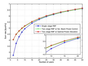
Fig. 3. Sum rate versus the number of users for Iterative Beam Power Allocation and Optimal Power Control with M = 2 transmit antennas, SNR = 10 dB, and Doppler shift  $f_D = 60$  Hz. Use of suboptimal iterative algorithm results in negligible loss compared to the optimal solution.
