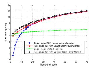
Fig. 5. Sum rate versus the number of users for On/Off Beam Power Control with M = 2 transmit antennas and SNR = 20 dB. On/Off beam power control switches to TDMA mode at low K, and strategy 4 gives almost same performance as strategy 3 without the additional feedback.
