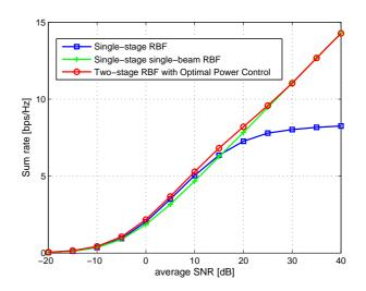
Fig. 2. Sum rate versus average SNR for Optimal Beam Power Control (strategy 3) with M = 2 transmit antennas, K = 10 users, and Doppler shift  $f_D = 60$  Hz. Beam power control circumvents the interference-limited behavior of RBF, achieving a linear sum-rate growth at high SNR.
