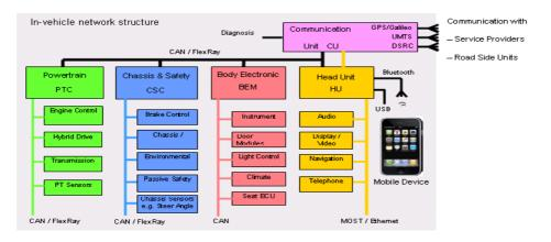
Figure 1: On-Board Reference Architecture [1]
