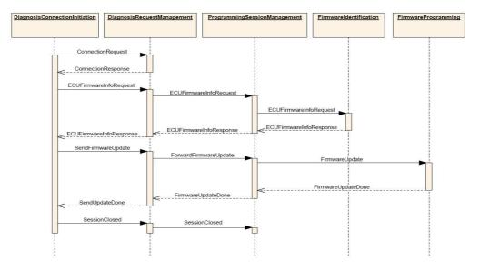
Figure 3: Functional View of Firmware Flashing Process
