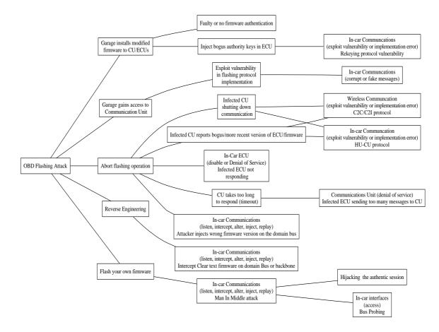
Figure 2: Attacks on Firmware Flashing Process [2]
