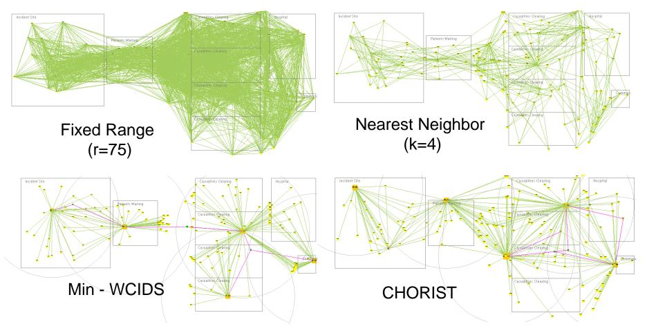
Aschenbruck et al. realistic model for node distribution over disaster area scenarios, based on a real based on a real maneuver simulation
