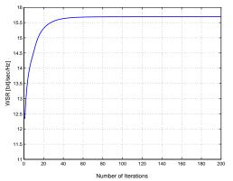
Fig. 4: Convergence behavior for a 3-user MIMO IFC with  $M_k = N_k = 4 \ \forall k$  at SNR=5dB
