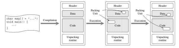
Figure 2: Overview of proposed on-the-fly (un)packing scheme (cross-hatched regions are packed; white regions inside the cross-hatched regions are not)
