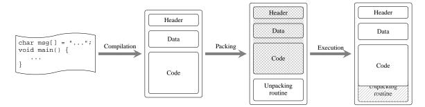
Figure 1: Overview of the traditional (un)packing scheme (cross-hatched regions are packed)
