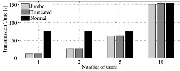
Fig. 6. Transmission time for Jumbo, *truncated* Jumbo and normal frames as a function of the number of users served.
