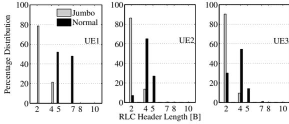
Fig. 5. Comparison of RLC Header length expressed in Bytes between Jumbo (gray bars) and normal (black bars) frames for the 450 MB file delivery.
