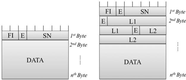
Fig. 2. RLC PDU example: 1 single SDU (left), 2 concatenated SDUs (right).
