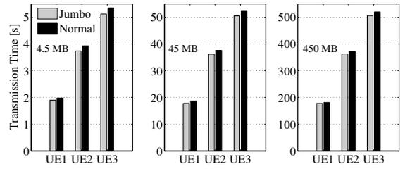
Fig. 3. Transmission time of three files with different sizes ( $\{4.5, 45, 450\}$  MB) for three users. Gray and black lines represent Jumbo and normal frames, respectively.
