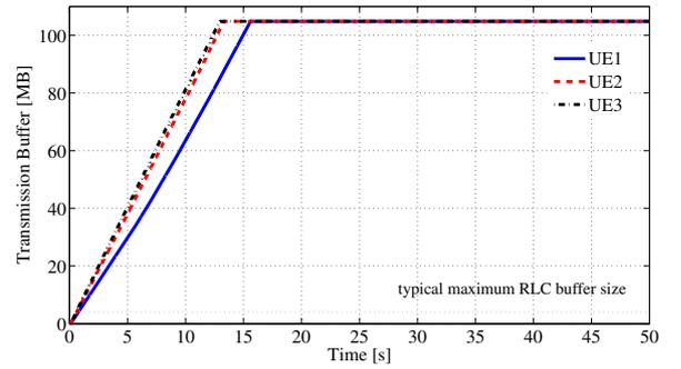
Fig. 7. Status of the RLC transmission buffer for Jumboframes transmissions. The typical size of the buffer is depicted for comparison.
