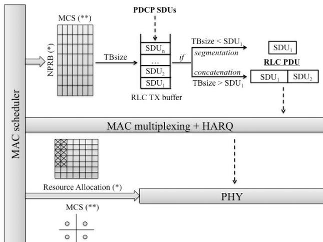
Fig. 1. Overview of the Radio Access mechanisms involved for Jumboframes transmissions in LTE networks.
