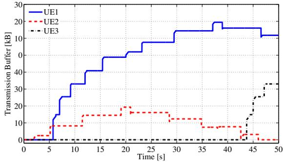
Fig. 9. Status of the RLC transmission buffer for *tuned* frame transmissions during the file delivery.
