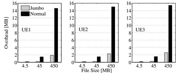
Fig. 4. Total overhead sent during the transmission of the 450 MB file for Jumbo and normal frames.
