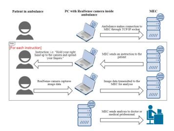
Fig. 2. High-level architecture for TeleStroke Assessment service.
