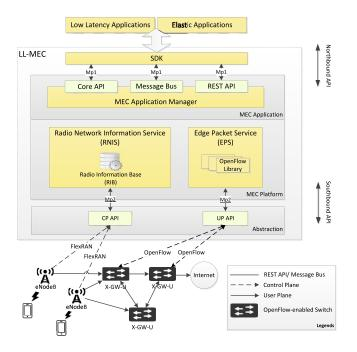
Fig. 5. High-level schematic of LL-MEC.
