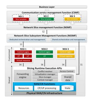
Fig. 3. RAN and CN runtime slicing system.
