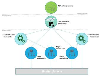
Fig. 6. P&P microservices architecture.
