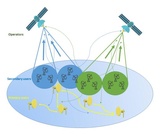
Fig. 1: A multi-operator CogSat communication system.
