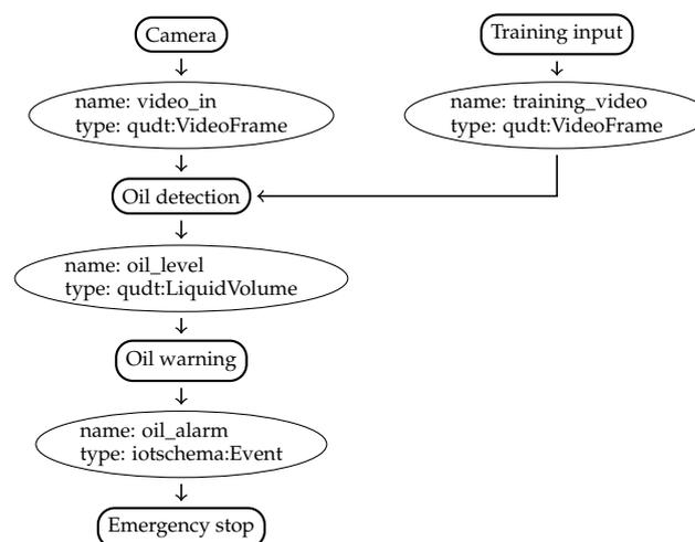
**Figure 2.** A simple oil leak detector recipe.
