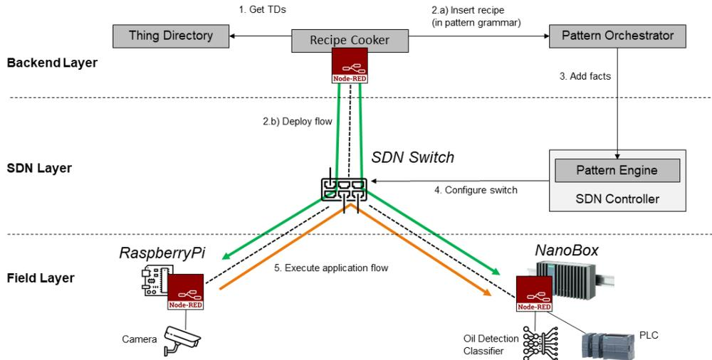
Figure 8. Setup of the oil leakage detection application.
