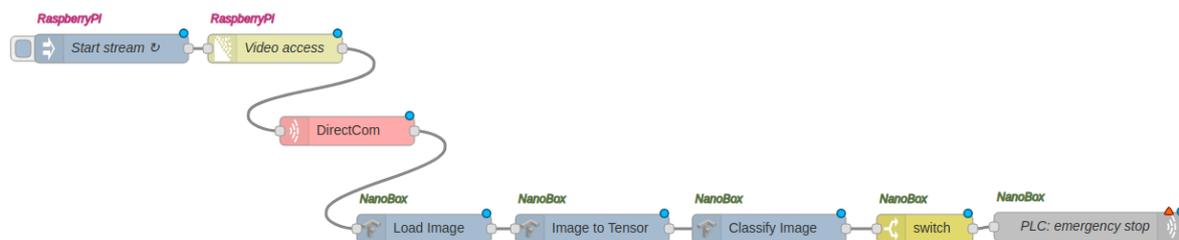
Figure 7. IoT application flow for oil leakage detection.
