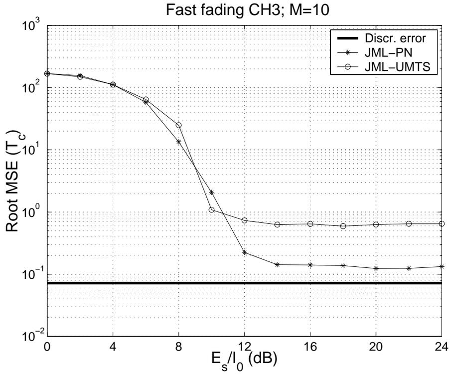
Figure 10: RMSE with fast fading CH3 vs.  $E_s/I_0$  for UMTS and PN sequences and  $M = 10$  accumulated bursts
