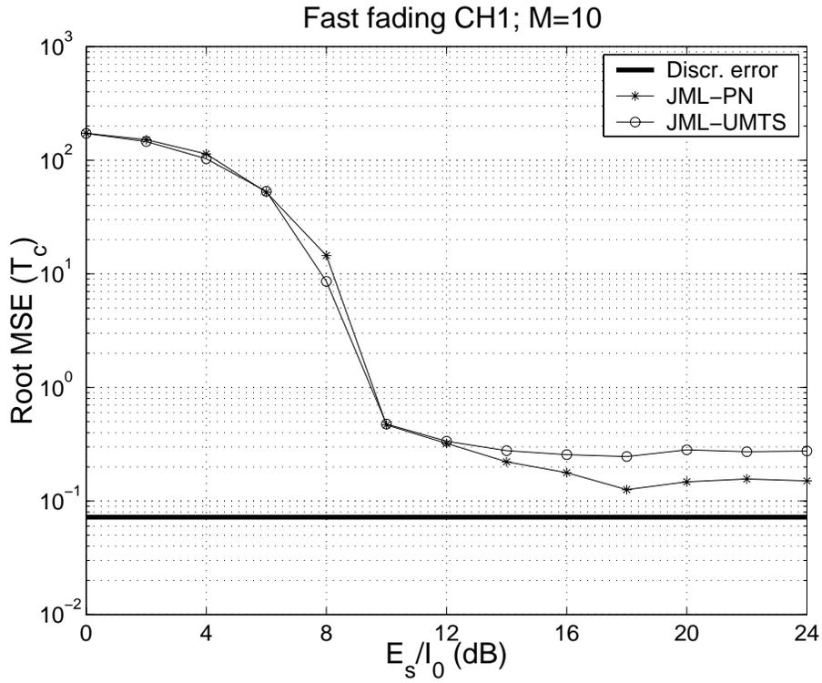
Figure 9: RMSE with fast fading CH1 vs.  $E_s/I_0$  for UMTS and PN sequences and  $M = 10$  accumulated bursts
