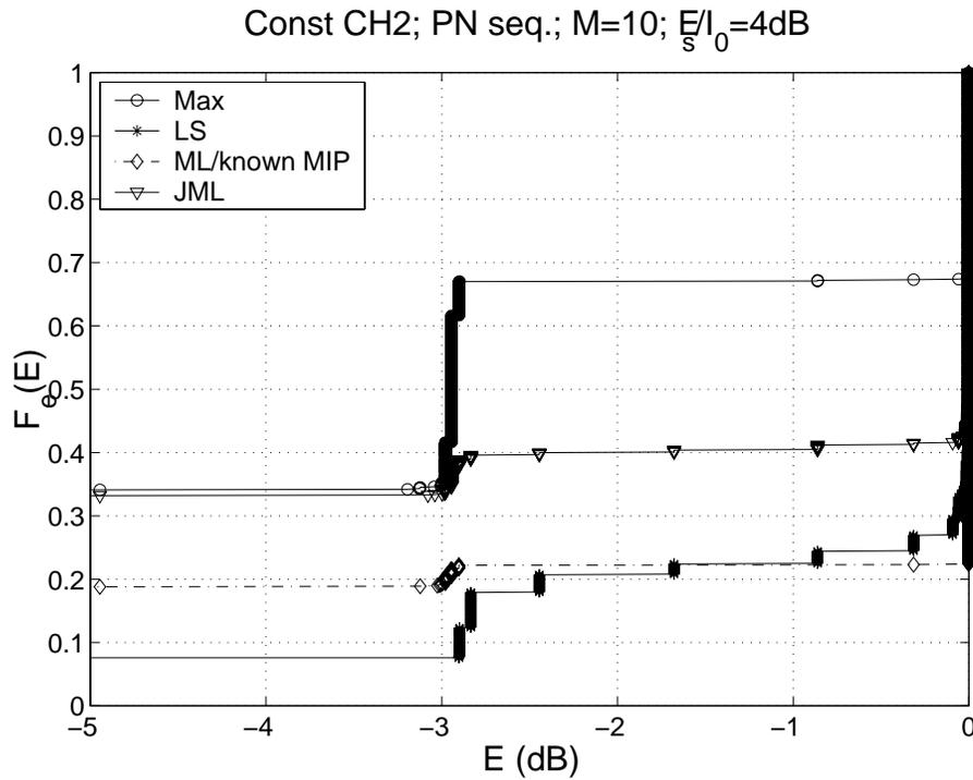
Figure 5: CDF with constant CH2 for  $E_s/I_0 = 4$  dB and  $M = 10$  accumulated bursts
