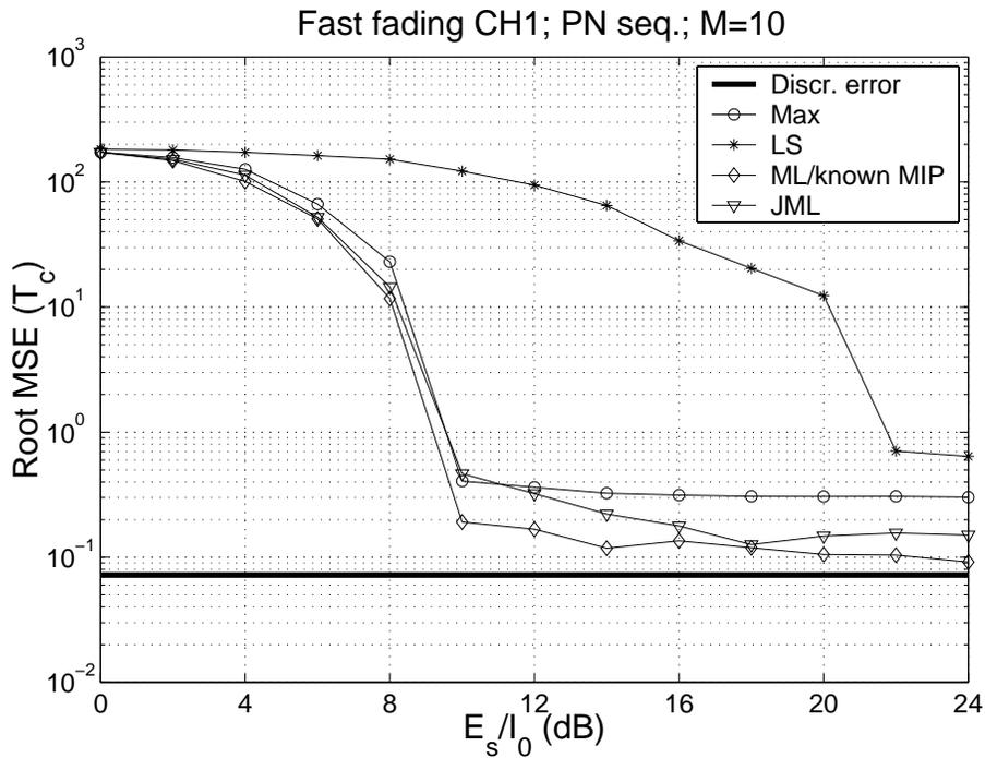
Figure 2: RMSE with fast fading CH1 vs.  $E_s/I_0$  for  $M = 10$  accumulated bursts
