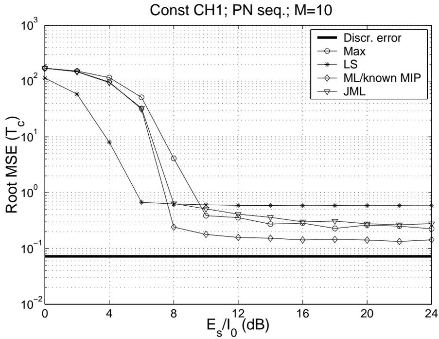
Figure 1: RMSE with constant CH1 vs.  $E_s/I_0$  for  $M = 10$  accumulated bursts
