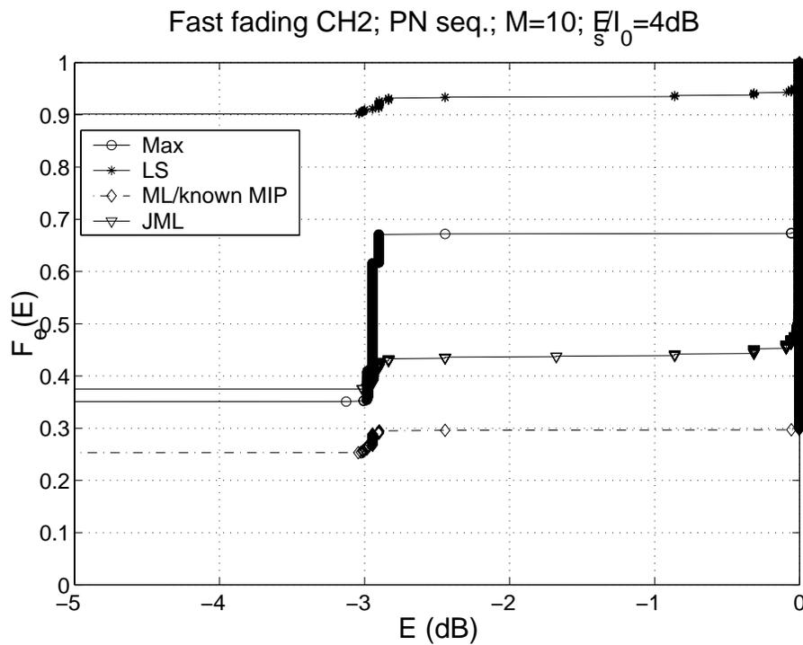
Figure 6: CDF with fast fading CH2 for  $E_s/I_0 = 4$  dB and  $M = 10$  accumulated bursts
