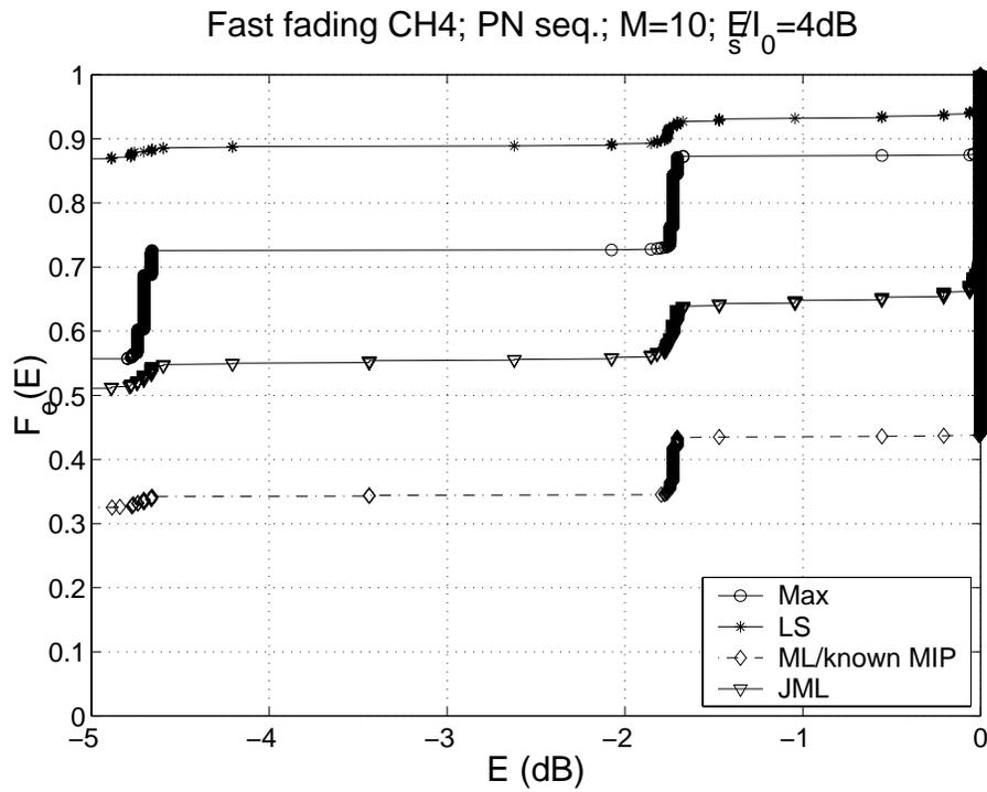
Figure 8: CDF with fast fading CH4 for  $E_s/I_0 = 4$  dB and  $M = 10$  accumulated bursts
