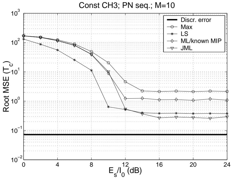
Figure 3: RMSE with constant CH3 vs.  $E_s/I_0$  for  $M = 10$  accumulated bursts
