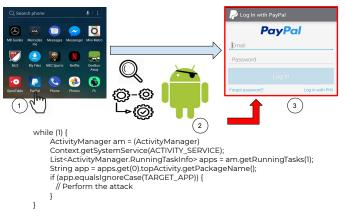
Fig. 1: Anatomy of a phishing attack.
