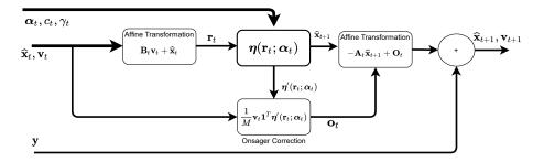
Fig. 1. Block diagram representing one iteration of LAMP-SBL.
