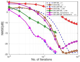
Fig. 3. NMSE versus the number of iterations/layers of the DNN, comprising (a) comparison with state-of-the art approaches; (b) for matrices with different condition numbers; and (c) with mismatched measurement matrices.
